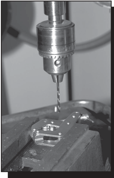
Figure 7—Using a \frac{1}{8} -inch drill bit, drill into the clamp pin to a depth of \frac{1}{4} inch. Turn the clamp over, secure it in the vise, and repeat the process. This provides a guide hole for the next step.
