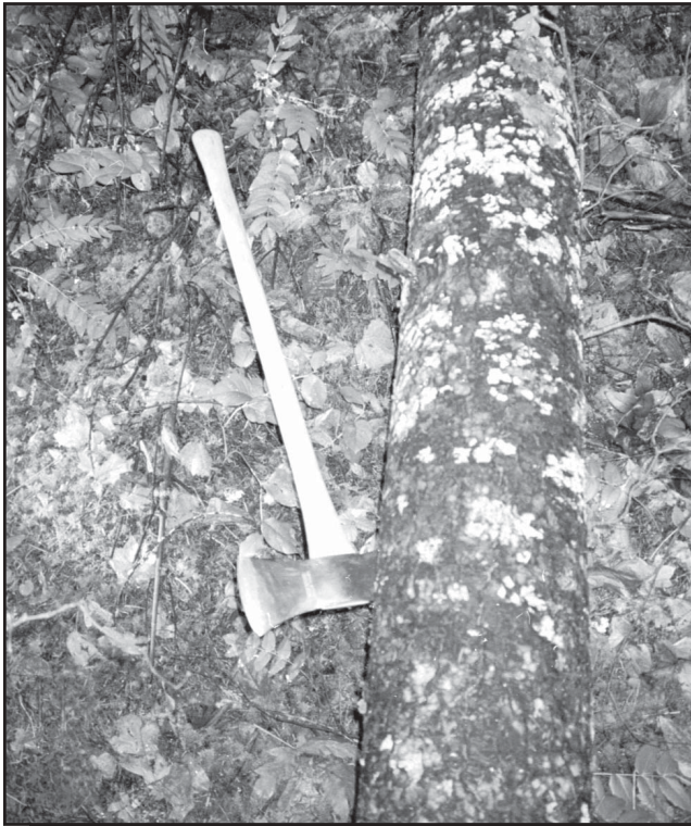
Figure 14—Insert the blade of the ax parallel to the log with the handle between 30 and 45 degrees to the log.
