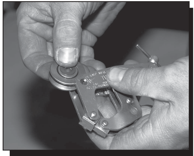
Figure 10—Insert the steel pulley and the two disc springs between the side plates of the clamp.
