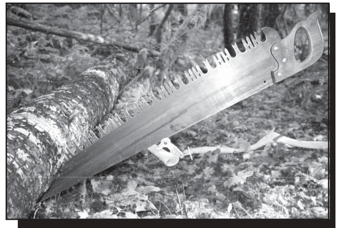
Figure 1—The underbuck supports the back of the crosscut saw and provides leverage for making cuts from the bottom of a log.
